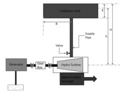
Fig. 3. Schematic Diagram of the Proposed system
