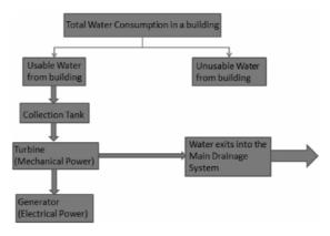
Fig. 2. Process of Extracting Energy from Grey Water
