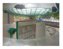
Fig. 4. Baffles within the Primary Settling tank
